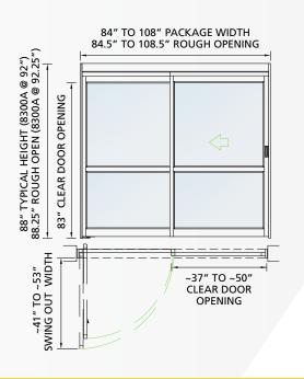
ProCare 8300: 2-panel manual sliding door with full swing out. Widest clear door opening in the industry, at 44.2" for on an 8' door.
