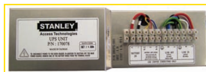
Uninterrupted Power Supply (UPS)
