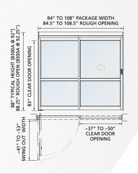
ProCare 8300: 2-panel manual sliding door with full swing out. Widest clear door opening in the industry, at 44.2" for on an 8' door.
