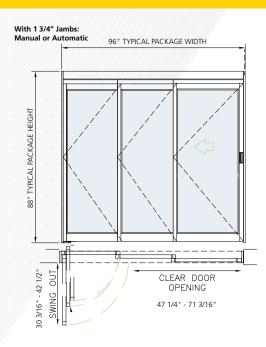
ProCare 8500: The latest ICU door in the ProCare Series, the 8500 offers the widest opening to allow for seamless patient and equipment movement without needing breakout. Available in automatic (8500A) or manual (power assist). The 8500A easily switches between manual and automatic mode. With the same size header utilized for both manual and automatic applications, site lines through the facility are maintained for an improved aesthetic.
