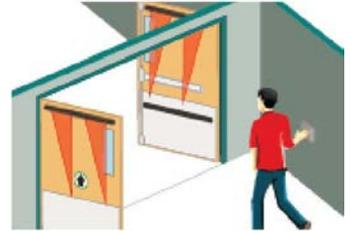
The M-Force™, Magic-Swing™ and Magic-Access™ operators are power-open, spring-close operators that have built-in emergency door release capabilities with controlled swing door return. Spring energy closes the door, with the speed controlled by using the motor as a dynamic brake.
